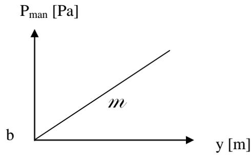
$$P_{\text{man}}[\text{Pa}] = m \left[ \frac{\text{Pa}}{\text{m}} \right] y [\text{m}] + b [\text{Pa}]$$
